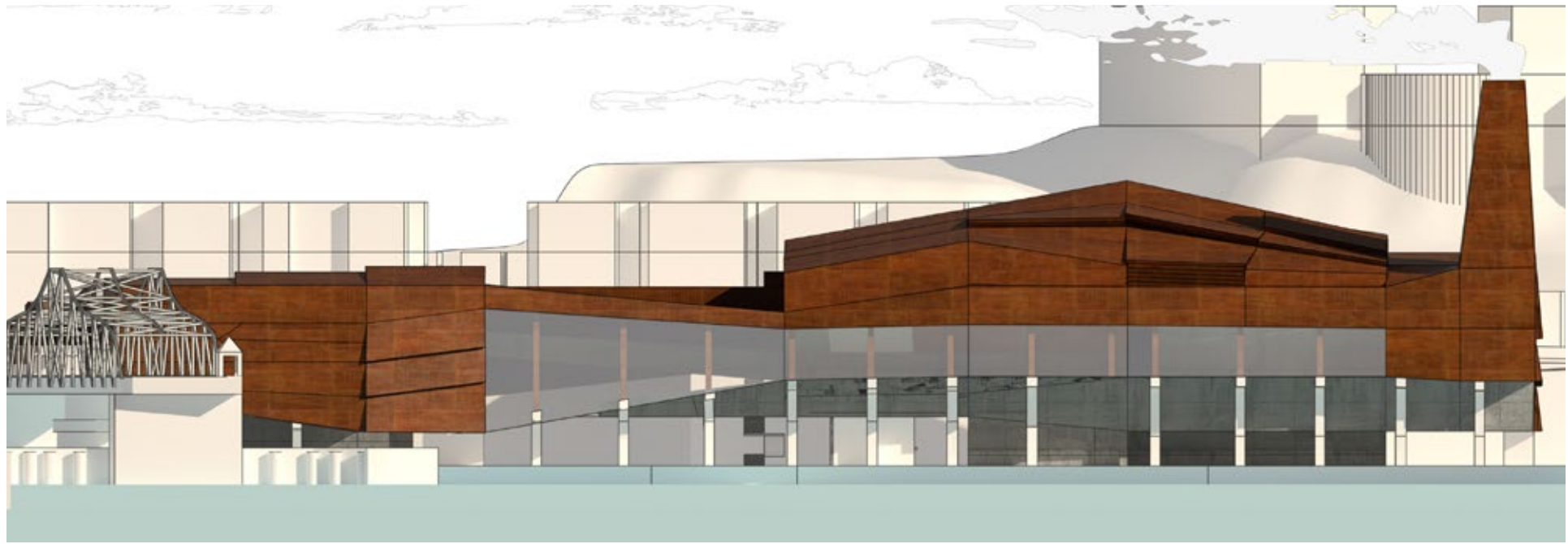
Elevation - The façade of the building is composed of copper panels, glazing, and louvers. The louvers are strategically placed to enhance ventilation.
